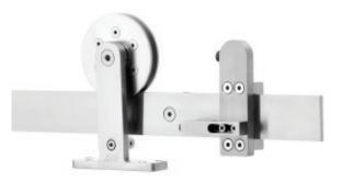
Crowder Flat Track 200 series features our classic top mount hangers for an ultra-modern look. 4" [101.6 mm] Delrin wheels combined with our precision ball bearings provide extremely smooth and quiet door operation. The Catch'N'Close closing system gently guides the door into position without any assistance. The precision-machined 304 stainless steel solid flat track and hardware are polished to a satin finish.
